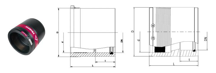
PE 100 Maximum permissible test pressure 0.5 bar to DIN EN 1610
