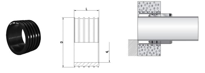
PE 100 Maximum permissible test pressure 0.5 bar to DIN EN 1610
